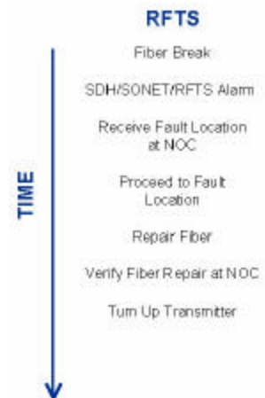
Typical workflow in the event of a catastrophic network fault with an RFTS
